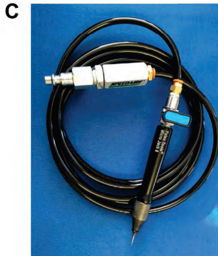
FIGURE 2.2. Tools used for preparation of the two specimens (MPC-D 102/111 and MPC-D 100/203) in this study. A , S30-40-3 from Seowon Compressor; B , ME-9100 from PaleoTools®; C , Micro Jack 6 from PaleoTools®. Not to scale.
